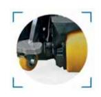
TRACTION AND STABILITY: Structure with 5 contact points and shock-absorber system for perfect grip by the driving wheel in case of floor irregularities. AC traction drives offer maximum responsiveness in starting and during braking.
